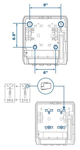
**Direct Mount:** Position unit on wall so that the top is level. Use key to open front cover and mark screw locations where indicated with circles. Secure unit to wall with four anchored screws appropriate to the type of wall in locations previously marked.
