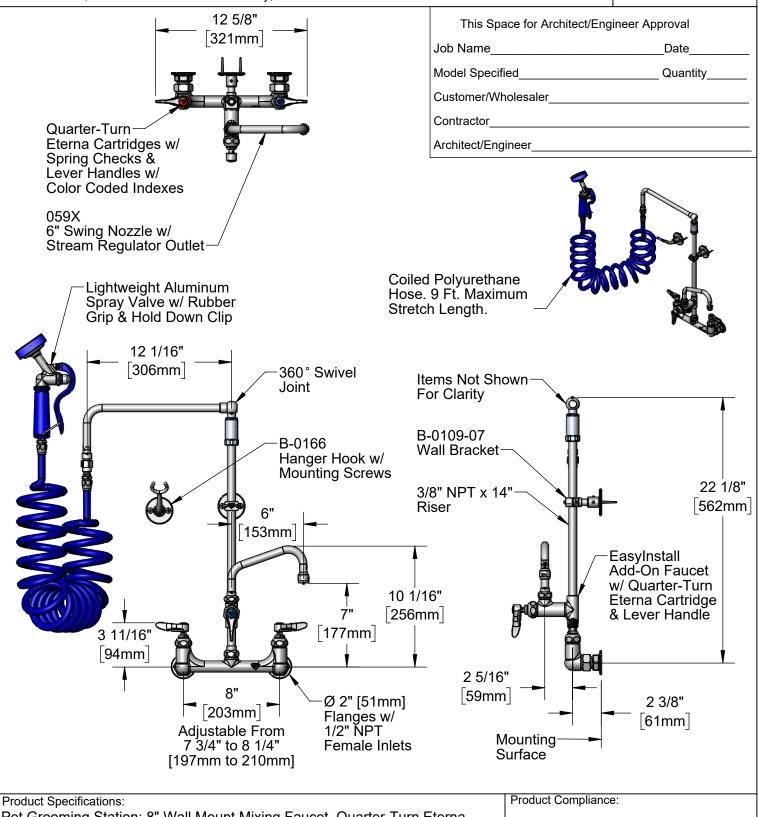
Pet Grooming Station: 8" Wall Mount Mixing Faucet, Quarter-Turn Eterna Cartridges w/ Spring Checks, Lever Handles, Add-On Faucet, 6" Swing Nozzle w/ Stream Regulator Outlet, Overhead Swivel Arm, 9' Coiled Hose w/ Angled Aluminum Spray Valve, Wall Bracket, Hanger Hook & 1/2" NPT Female Inlets
