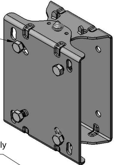
Both Upper & Lower C-Clips Must Be Installed Immediately after Hose Reel Installation
