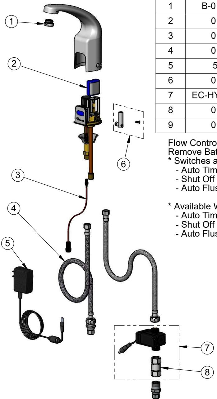
Flow Control Switches are Located Behind the Sensor.
