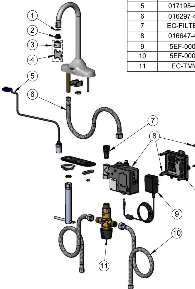
A Maximum of (8) ChekPoint Faucets can be Hardwire Connected and Powered by EC-HARDWIRE ChekPoint Hardwire AC Transformer. (Sold Separately)
