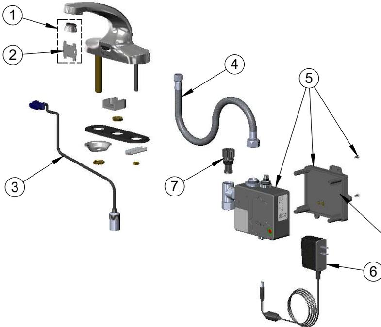
A Maximum of (8) ChekPoint Faucets can be Hardwire Connected and Powered by EC-HARDWIRE ChekPoint Hardwire AC Transformer. (Sold Separately)
