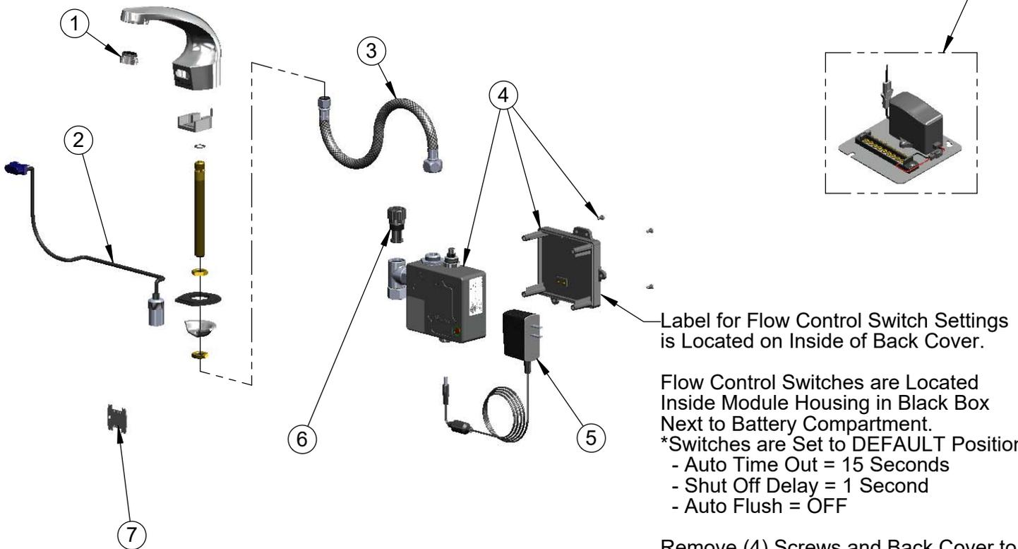
Label for Flow Control Switch Settings is Located on Inside of Back Cover.
