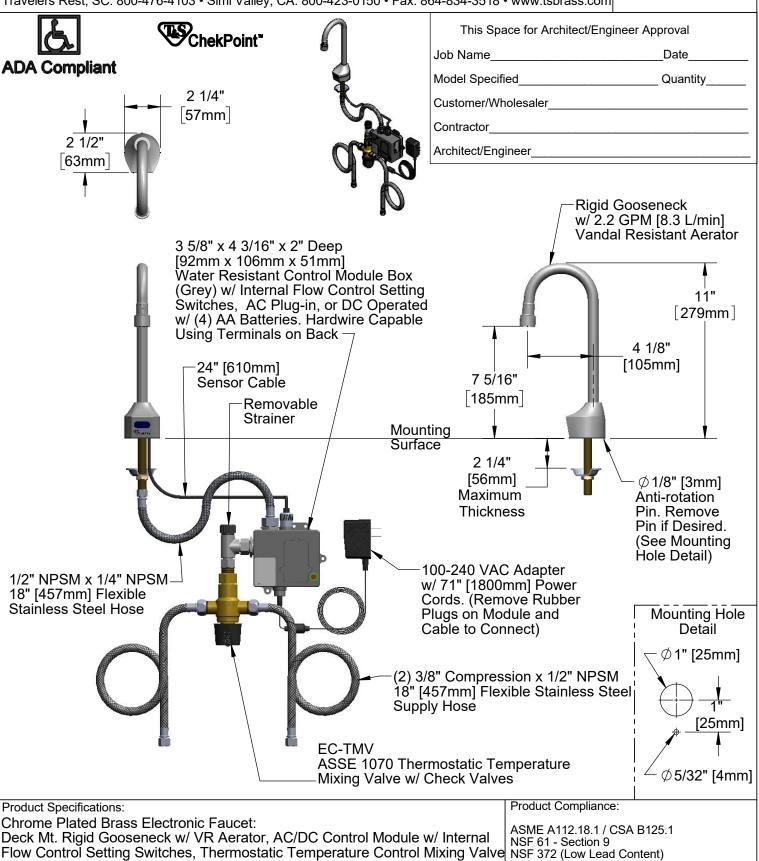
Flow Control Setting Switches, Thermostatic Temperature Control Mixing Valve
