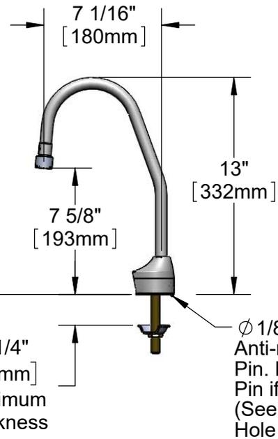
Ø 1/8" [3mm] Anti-rotation Pin. Remove Pin if Desired. (See Mounting Hole Detail)
