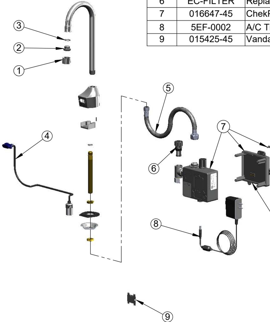
A Maximum of (8) ChekPoint Faucets can be Hardwire Connected and Powered by EC-HARDWIRE ChekPoint Hardwire AC Transformer. (Sold Separately)
