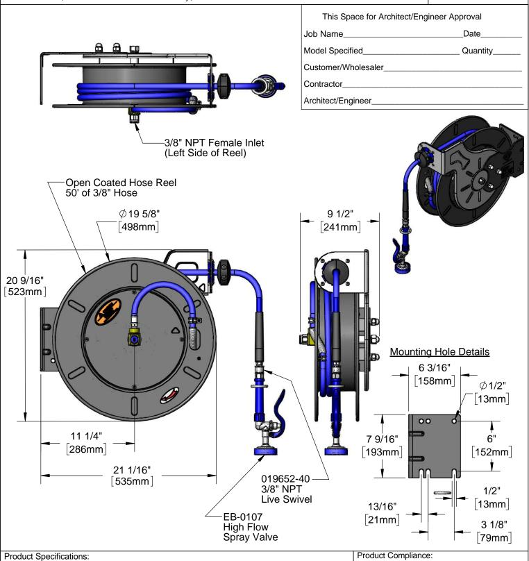
3/8" x 50' Open Coated Reel & High Flow Spray Valve & Swivel
