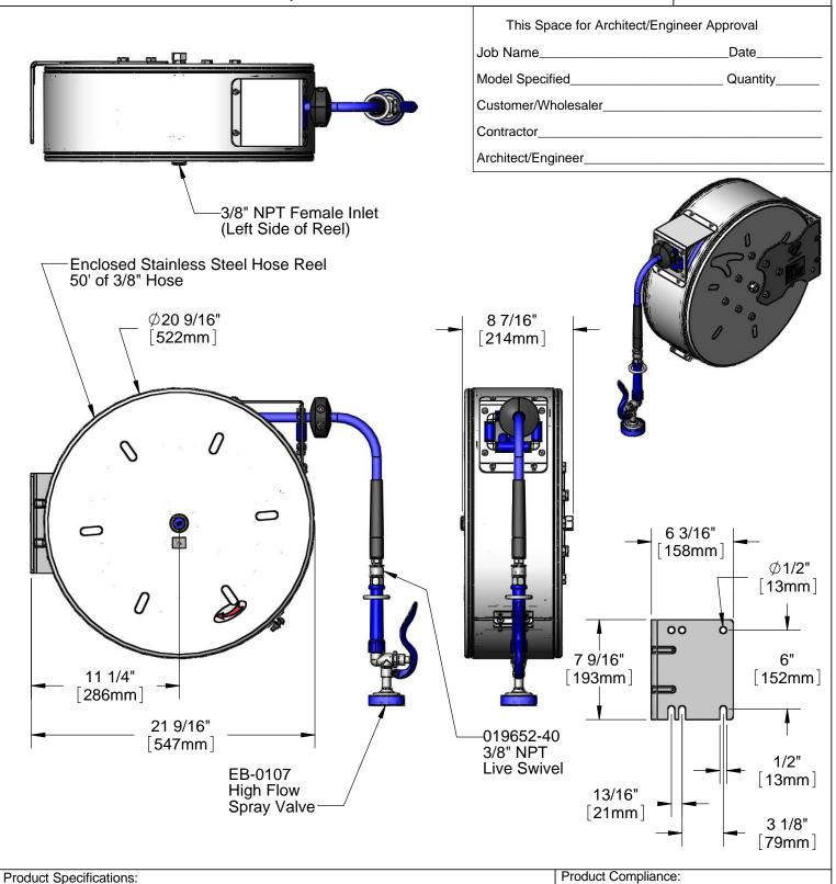
3/8" x 50' Enclosed Stainless Steel Reel w/ High Flow Spray Valve & Swivel
