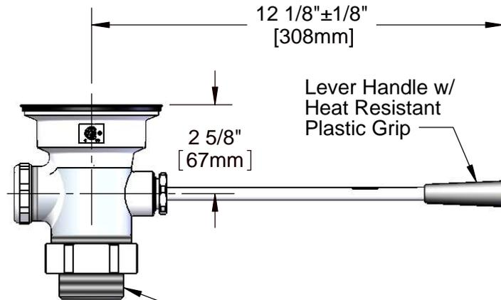
Adapter Converts 2" NPT Male to 1 1/2" NPT Male. Remove Adapter When 2" NPT Male Thread is Needed.
