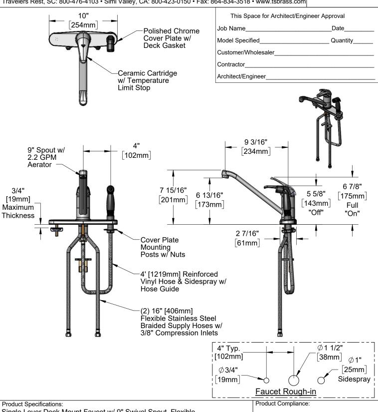
Single Lever Deck Mount Faucet w/ 9" Swivel Spout, Flexible Supplies, 10" Cover Plate w/ Sidespray Opening, 48" Sidespray, & Ceramic Cartridge w/ Temperature Limit Stop
