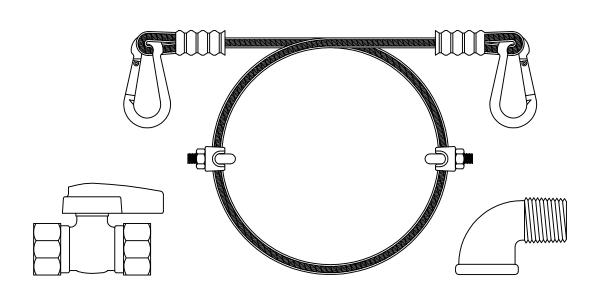
INSTALLATION KIT CONTAINS (1) EACH: RESTRAINING CABLE, STREET EL, BALL VALVE
