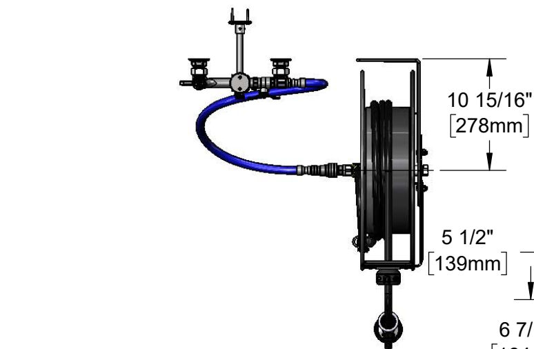
B-0963 Continuous Pressure Vacuum Breaker w/ Integral Check Valve
