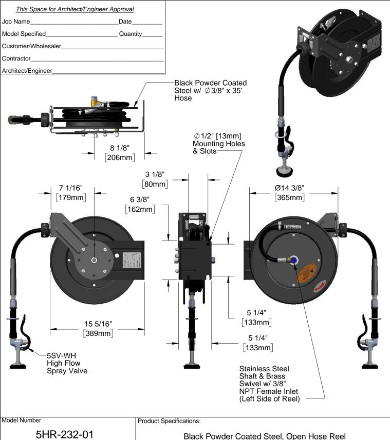
Black Powder Coated Steel, Open Hose Reel w/ Ø3/8" x 35' Hose & High Flow Spray Valve **Product Compliance:** EPAct 2005 Non-Compliant (PRSV) NSF 61 Exempt (Non-Potable) 2 Saddleback Cove, P.O. Box 1088 Travelers Rest, South Carolina 29690 Phone: 800.891.4808 Fax: 800.868.0084 equip
