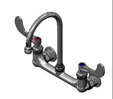
Swivel Gooseneck w/ 2.2 GPM Laminar Flow Device Converts to Rigid w/ 014200-45 Lock Washer (Included). Quarter-Turn Cerama Cartridges w/ Check Valves & 4" Wrist Swivel Joint Action Handles w/ Color Coded Indexes 5 5/16" [134mm] Ø 2" [51mm] 8" Flanges w/ [203mm] 1/2" NPT Adjustable From Female Inlets 7 3/4" to 8 1/4" [197mm to 210mm]
