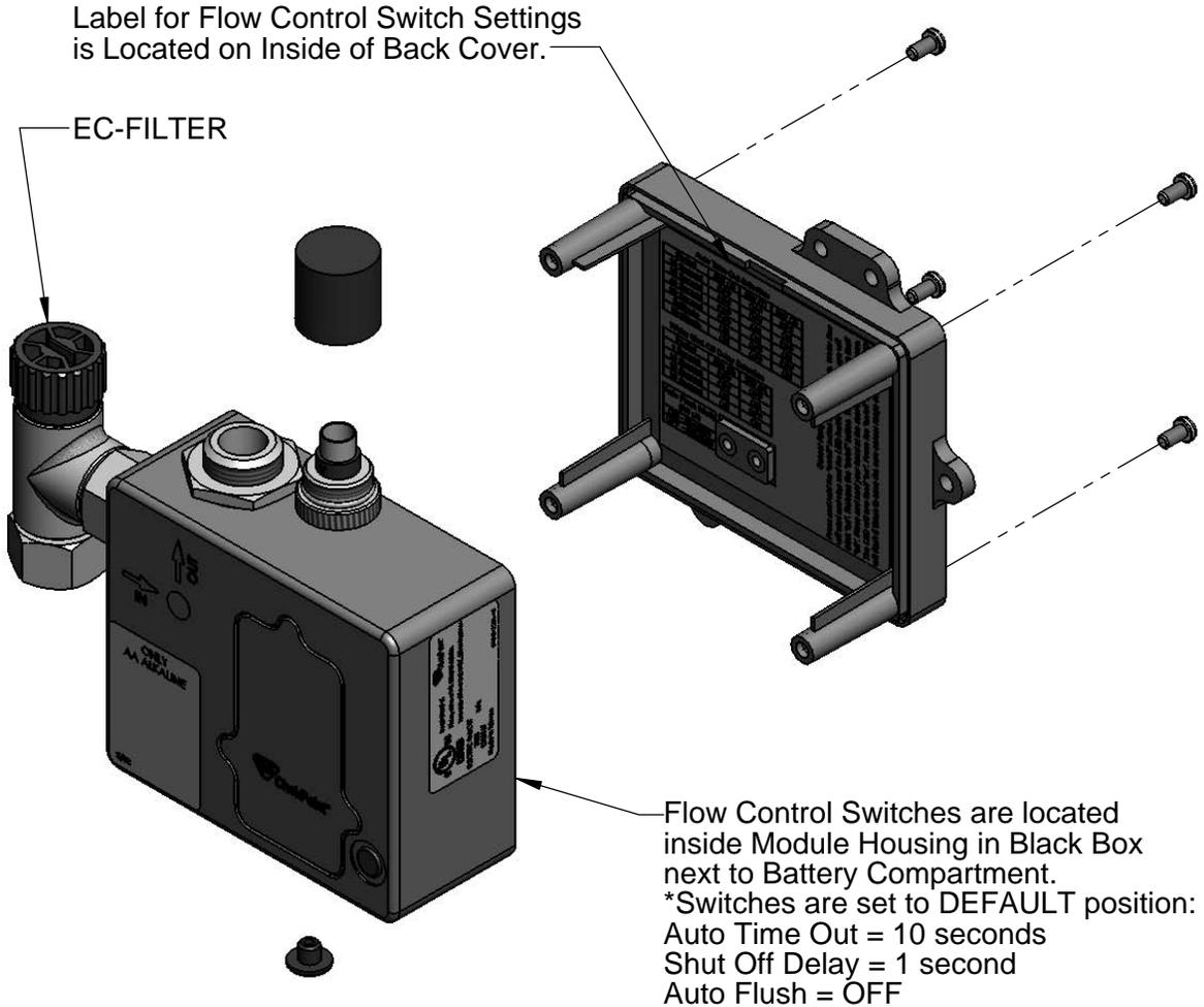
Remove (4) screws and back cover to access switches.
