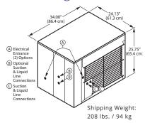
208-230/60/1standard. 208-230/60/3 HACR-type circuit breakers can be used in place of fuses.
