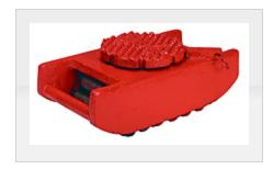
HeviMovers<sup>™</sup> are made with precision ground and hardened steel rollers that form an endless chacentral load-bearing plate in the frame. Weight of the load is transferred directly from load-bearing eliminates axle friction and requires less power to start and move the load. HeviMovers<sup>™</sup> roll easily floor areas to reduce possible damage to goods.
