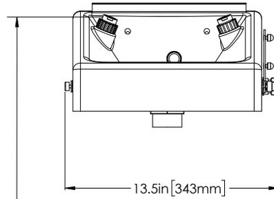
TO COMPLY WITH ANSI Z358.1: EYE/FACE WASH NOZZLES SHALL BE POSITIONED 33 in [83.8 cm] TO 45 in [114.3 cm] FROM STANDING SURFACE. FLUSHING FLUID SHALL NOT EXCEED 8 in [20.3 cm] ABOVE NOZZLES.
