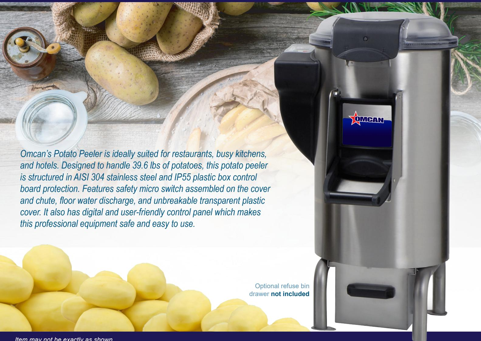
Omcan's Potato Peeler is ideally suited for restaurants, busy kitchens, and hotels. Designed to handle 39.6 lbs of potatoes, this potato peeler is structured in AISI 304 stainless steel and IP55 plastic box control board protection. Features safety micro switch assembled on the cover and chute, floor water discharge, and unbreakable transparent plastic cover. It also has digital and user-friendly control panel which makes this professional equipment safe and easy to use.
