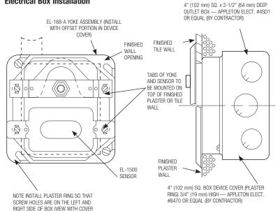
Position of Sensor Box can be raised or lowered 1" (25 mm) if in conflict with Handicap Grab Bars.
