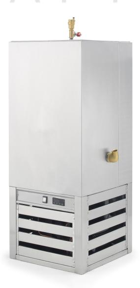
Water Chiller, 100 Liter Capacity (26.4 Gallons), Minimum Temperature of 2C° (36° F), Display in Celsius, Thermally Insulated, Closed Tank Cooling System with Tubes for Water Circulation, Equipped with Compressor, Air Valve, Purge Valve and Entry Cut-Off Valve, Outflow Equal to Inflow, 370 Watts, 208-240V/60/1P/2.1A, NEMA 6-15P, cETLus
