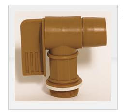
2" NPT polyethylene faucet produced from FDA approved material. Includes 3 EPDM sealing gaskets: thin, medium, thick. Good for viscous noncorrosive fluids.
