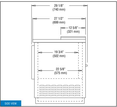
**IMPORTANT NOTE**: A <u>minimum clearance of 3" is required</u> on each side, front and rear of cabinet for optimum performance.
