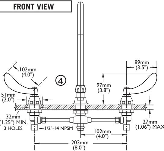
INLET FOR 3/8" OR 1/2" FLEXIBLE RISER OR 1/2-14 NPSM COUPLING NUT (NOT SUPPLIED)
