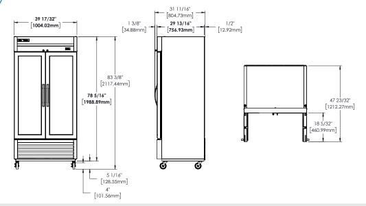
METRIC DIMENSIONS ROUNDED UP TO THE NEAREST WHOLE MILLIMETER
