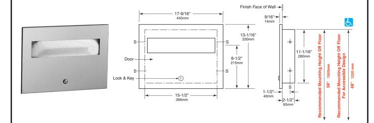
Rough Wall Opening 15-7/8" (405mm) wide 11-7/16" (290mm) high 2-3/4" (70mm) minimum recessed depth
