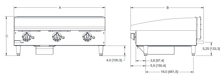
\*UNITS OPERATE ON NATURAL GAS OR PROPANE GAS 3/4" (1.9 cm) N.P.T. Male Gas Connection
