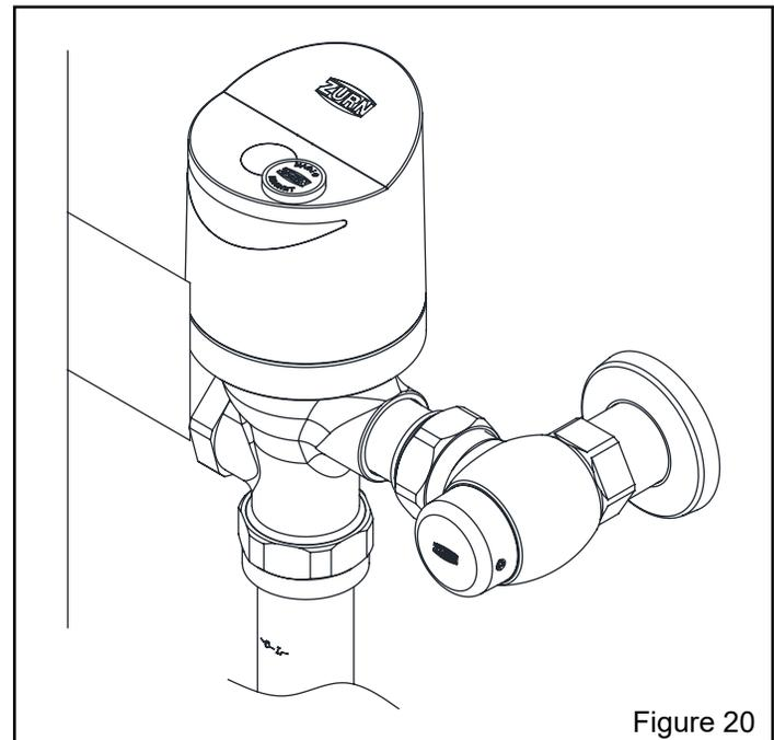
**⚠** While in range verification mode, test calibrated sensor range using targets of various material types/textures to ensure calibration accuracy. Verify that sensor range does not detect stall doors or other reflective surfaces.
