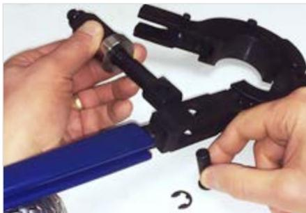
2. Push the pin out with the screw driver until you can grab it with your fingers, then remove the pin and screw/nut assembly from the tool.
