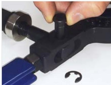
1. Clean the pin area of the tool with a brush and rag to remove any dirt and surface rust.
