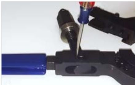
1. If necessary, remove existing E-Clip by prying it away from the pin with a flat head screw driver.
