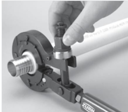
the tool jaws. Confirm the tool is at a 90° angle to the fitting and close jaw. Hand tighten the nut to hold fitting assembly in place.
