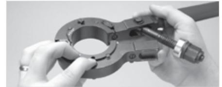
1. Open clamp, then press spring/pin with finger to disengage jaw retainer.
