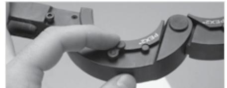
2. Continue to hold in the spring/pin, turn tool around and rotate jaw retainer clockwise until it clears the jaw and can rest on the tool. Remove jaw from tool.
