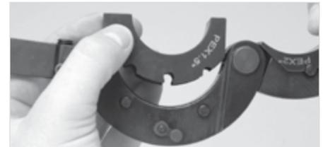
3. Insert new crimping jaw. Notches in jaw must align with pins on tool.
