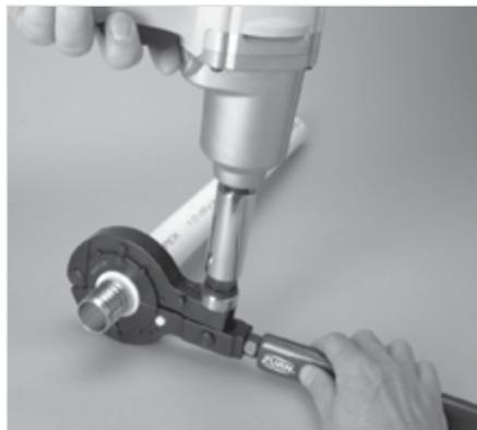
5. Drive the nut down with an impact wrench until blue LED light turns on.
