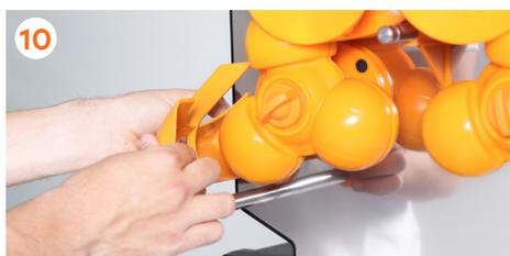
10 Pull off the peel ejectors.
