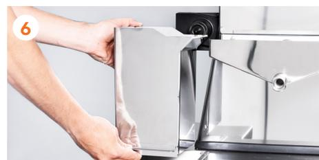
6 Remove the stainless-steel **peel guides**.
