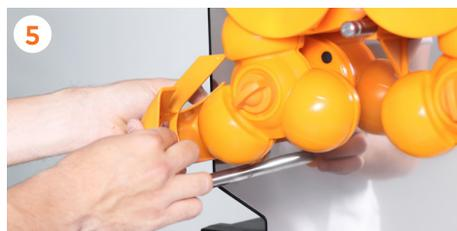
5 Pull off the peel ejectors.
