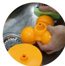
Cleaning of the machine and any of its removable parts must be done with a **sponge soaked in Citric Active soapy water**. Do not use scouring sponges that could scratch the surfaces.
