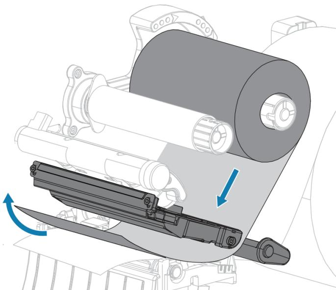
Wrap the ribbon around the core several times, and then rotate the spindle to tighten and align the ribbon.
