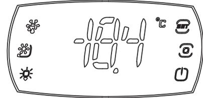
Always remember to calculate the differential if you change the minimum temperature setting. The cabinet temperature will fluctuate up to +7 degrees over your set minimum temperature as the compressor runs and shuts off. Setting the temperature too high will result in unsafe maximum temperatures and possible health code violations.
