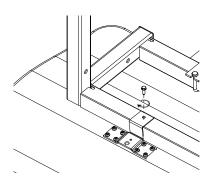
d. Now that the seat is installed, insert a self-drilling screw into the hole in the rear seat hook. One screw for each rear seat hook. Do not over tighten.
