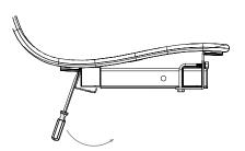
Screw drive shown prying rear seat hook on contour seat. above Same method used for flat bench.
