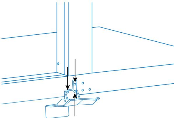
3. After installation, test the foot pedal. If the foot pedal position is not ideal, you can loosen the screws and adjust the position left and right as shown. Retighten the screws before use.
