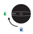
Step 4: Turn the gas valve counter clockwise to closed. (located on the gas cap).
