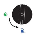
Step 4: Turn the gas valve clockwise to open. (located on the gas cap).
