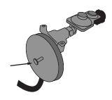
Step 5: Attach the LPG hose to both the generator inlet and the propane tank, then turn the tank on.
