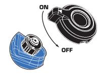
Step 6: Press the decompression valve on the regulator.
