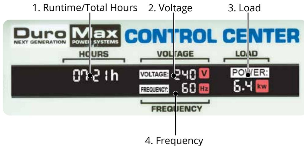
1. **Runtime/Total Hours** – This portion of the display will automatically switch between the current runtime and total runtime hours of the unit.
