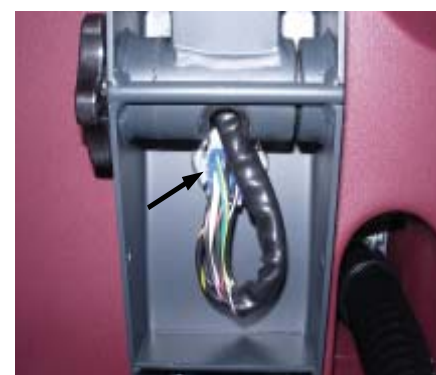
The wire harness must be aligned with the patterns on the connector to fit.
