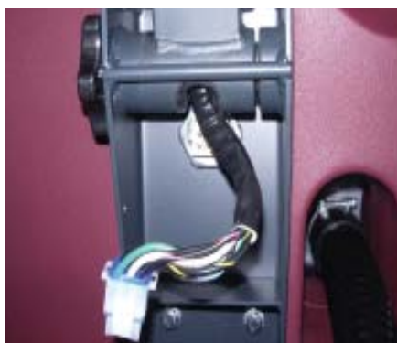
Attach the wire harness to the machine.
