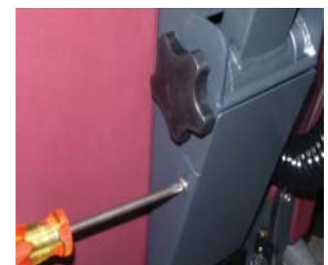
Screw the cover back with the 4 screws.
