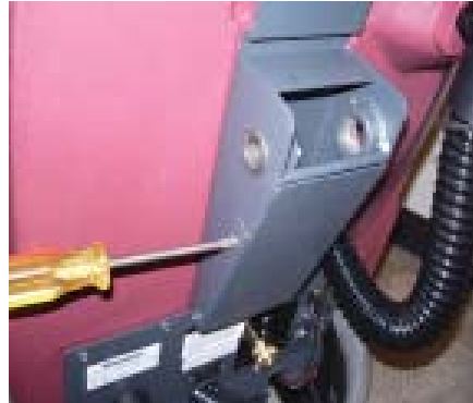
Use philips screwdriver to unscrew 4 screws and remove cover.
