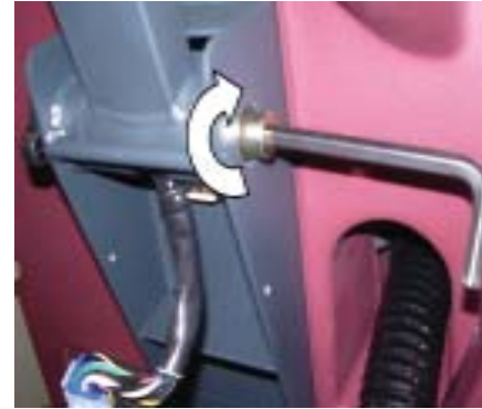
Insert handle assembly in between bushings. Insert the shoulder bolt through the bushing and screw into the handle assembly using supplied wrench.
