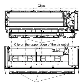
Clip on the bottom edge of the air outlet
