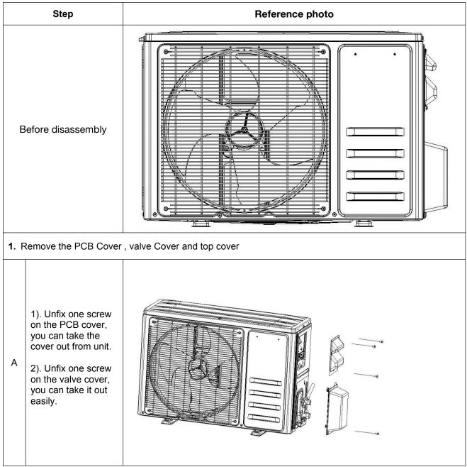
Unfix screws btw the top cover with front panel, left and right plate, then you can take the top cover out.
