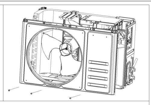
3: Disassemble the Left and Right plate.
