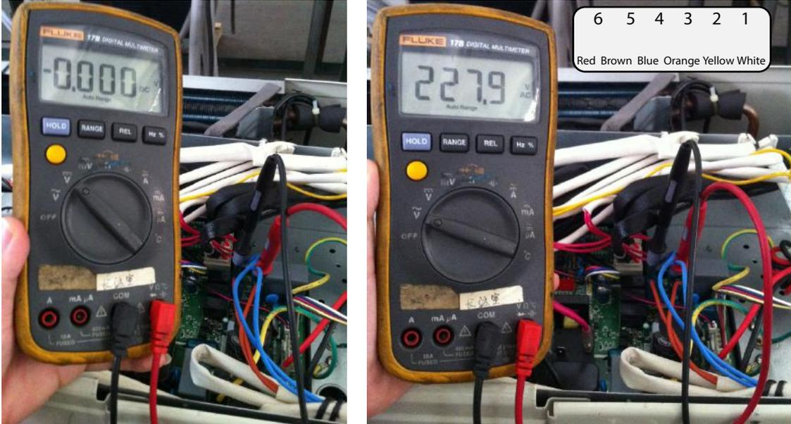
2. Turn off the power, and use a digital tester to measure the valve's resistance. The value should be 1.8~2.5 K $\Omega$ .
