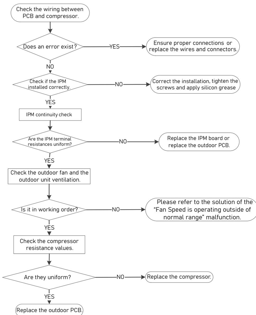
**Note:** For certain models, outdoor PCB cannot be removed separately. In this case, the outdoor electric control box should be replaced as a whole.
