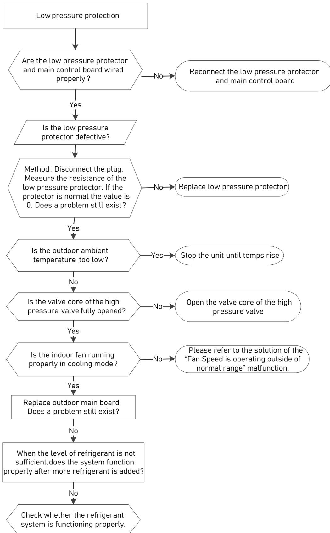
**Note:** For certain models, outdoor PCB cannot be removed separately. In this case, the outdoor electric control box should be replaced as a whole.
