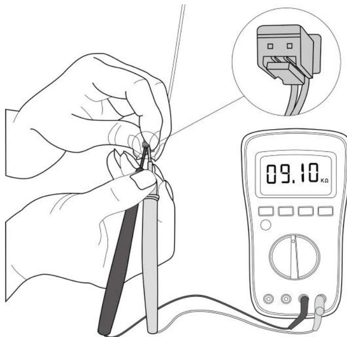
**Note:** For certain models, outdoor PCB cannot be removed separately. In this case, the outdoor electric control box should be replaced as a whole. This picture and the value are only for reference, actual appearance and value may vary. For certain models, outdoor unit uses combination sensor (T3, T4 and TP are the same of sensor).
