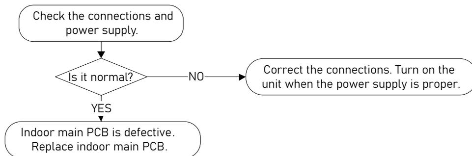
**Note:** E2/EH 02 zero crossing detection error is only valid for the unit with AC fan motors, for other models, this error is invalid.
