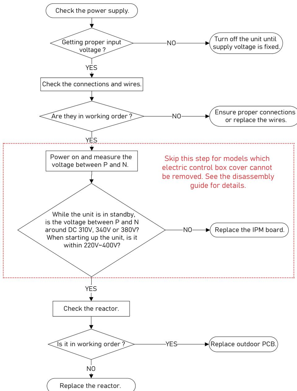
**Note:** For certain models, outdoor PCB cannot be removed separately. In this case, the outdoor electric control box should be replaced as a whole.
