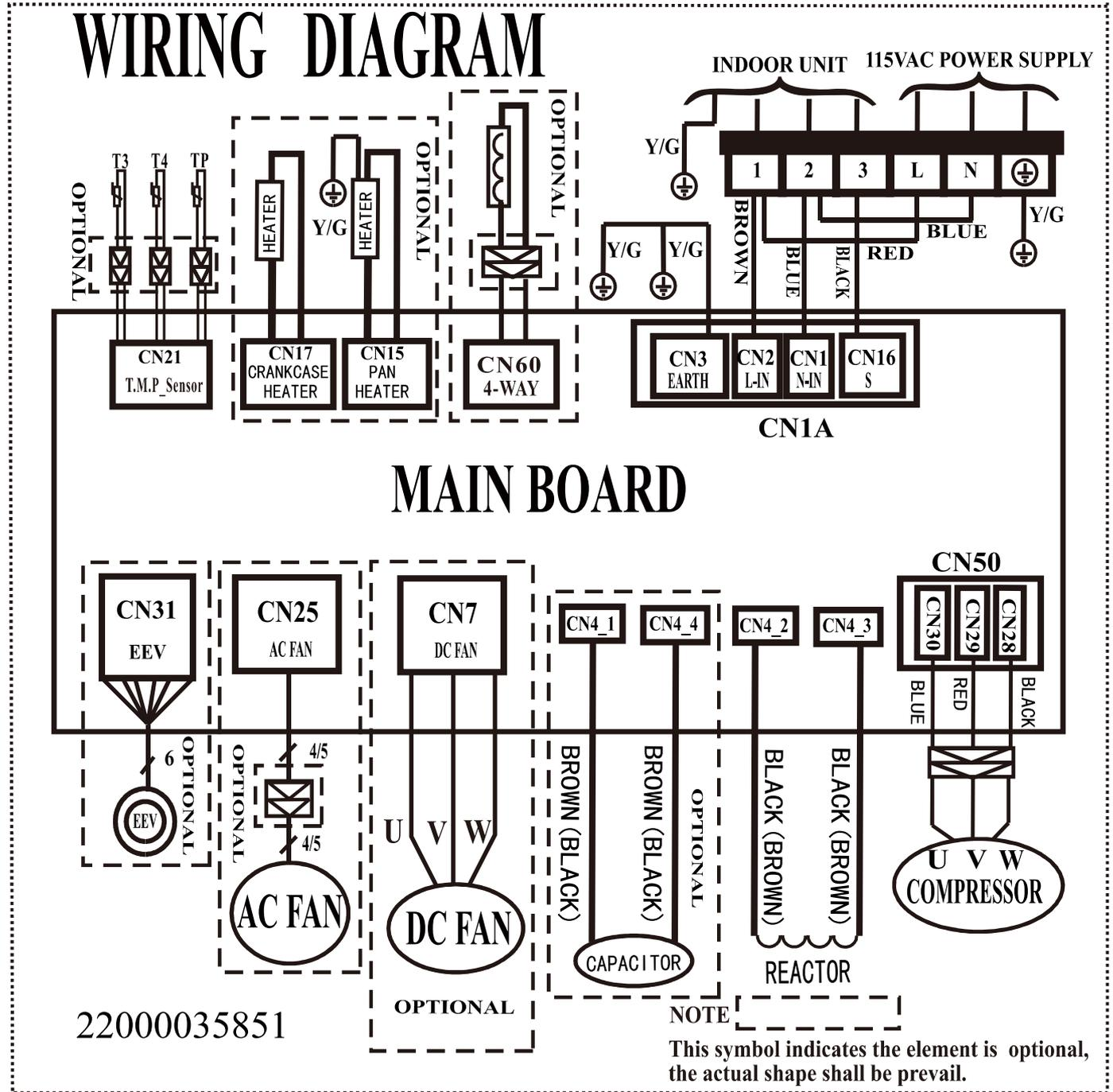
Outdoor Unit Wiring Diagram: 22000035853
