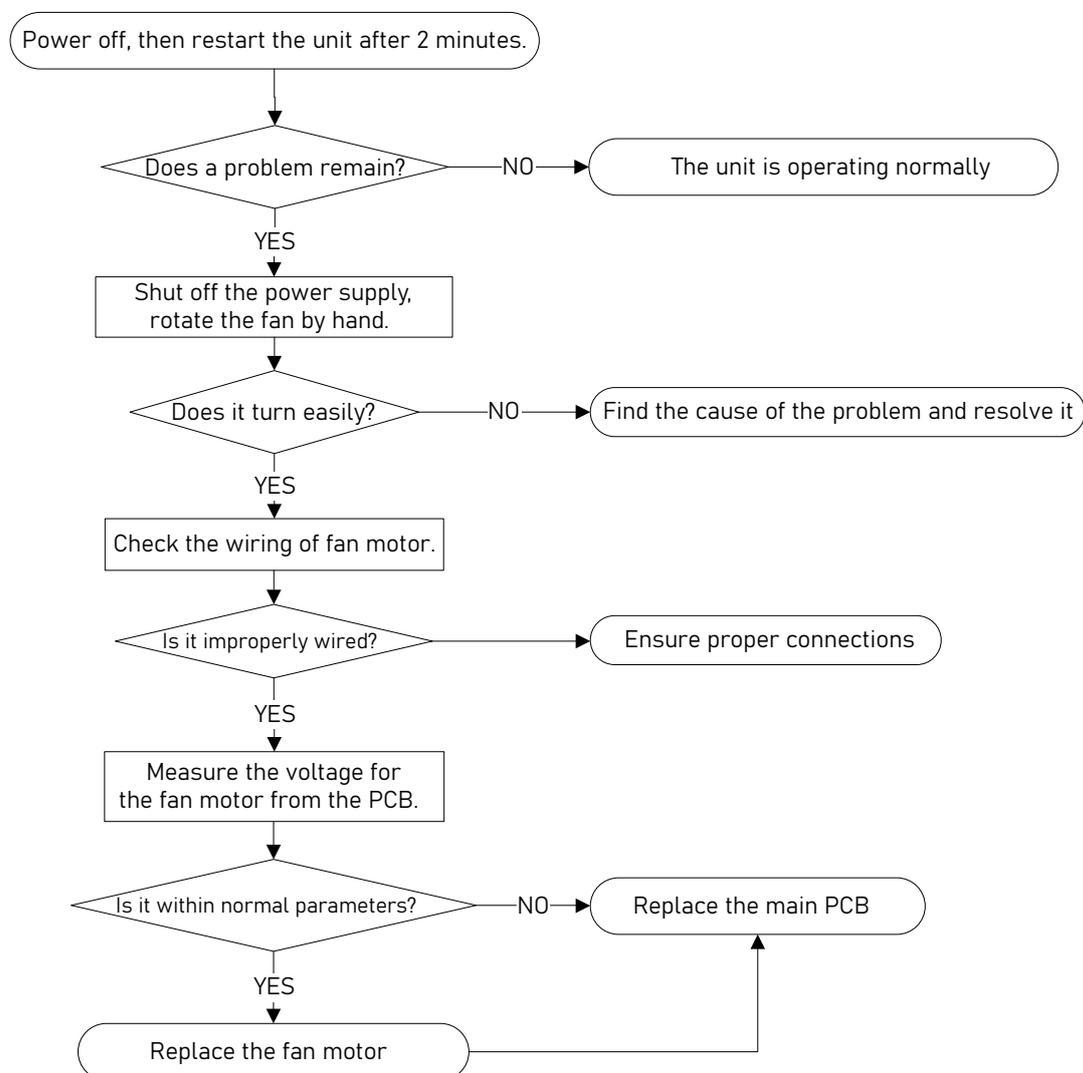
**Note:** For certain models, outdoor PCB cannot be removed separately. In this case, the outdoor electric control box should be replaced as a whole.
