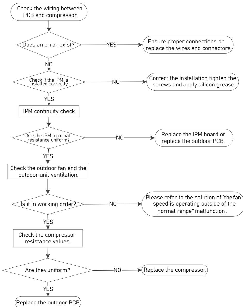
**Note:** For certain models, outdoor PCB cannot be removed separately. In this case, the outdoor electric control box should be replaced as a whole.
