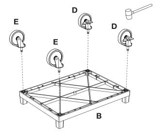
IMPORTANT: Flip shelf B, and lock the 2 locking casters **D** before assembling
