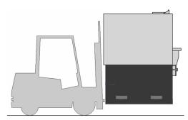
**1** Use a forklift (or pallet jack) to raise the oven using the front or rear forklift pockets.
