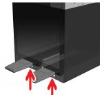
Make sure the Pallet Jack wheels do not contact the underside of the fork pocket when lifting to avoid damaging the stand.
