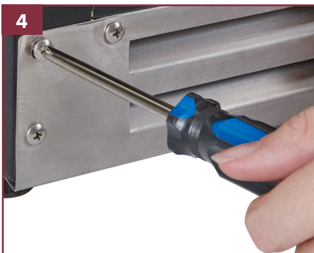
4. Remove the 3 screws on the left side of the kick plate.
