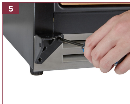
5. Rotate the lower hinge 90° counterclockwise and secure to the left side of the kick plate with 3 screws.
