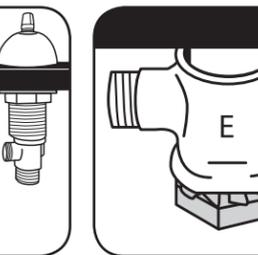
10. Install lockwasher and nut to the shank. Hand tighten.
