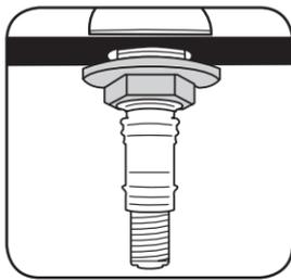
3. From below deck, use nut and metal washer to secure spout to deck. Hand tighten.
