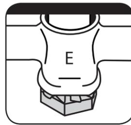
5. Install lockwasher and nut to the shank. Hand tighten.
