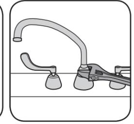
3. Place spout into stem. Tighten spout nut with wrench. Connect water supplies, flush line, and attach outlet.
