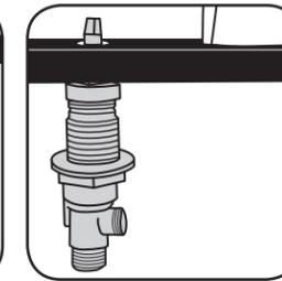
4. From below deck, align handles with deck holes. Push through deck hole and repeat with other side.
