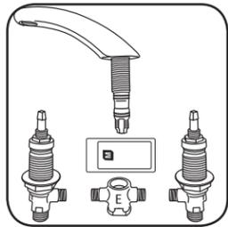
1. Using grease from supplied packet, lubricate the 4 o-rings on the spout shank and inside of center hub of undermount body.
