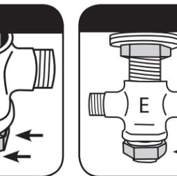
11. With a wrench, tighten center lower nut on shank and upper center nut.
