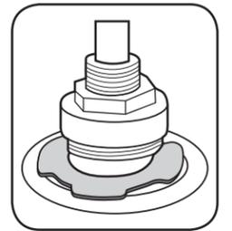
6. Slide a retaining clip on top of the sealing washer and into the groove of each cartridge housing.
