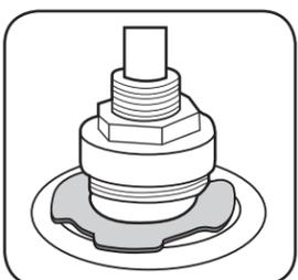
7. Slide a retaining clip on top of the sealing washer and into the groove of each cartridge housing.
