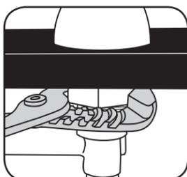
9. Below deck, hand tighten the flanged nuts and then with a wrench tighten 1/4 - 1/2 turn more.
