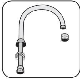
1. Remove outlet from spout. Place two split rings on spout near the base. Slide spout nut onto spout.
