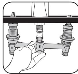
4. Align the undermount body (marked H & C for connections) with deck holes and shank. Push the center of the undermount body (E) onto shank. Be careful not to pinch o-rings.
