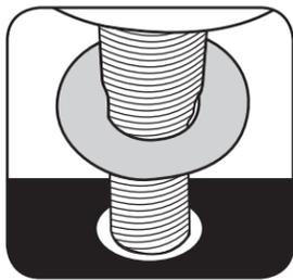
2. Slide the shank through the slim rubber washer and top center hole of deck.
