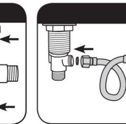
12. Connect left supply line to left handle and left side of water connector. Repeat with right supply line.
