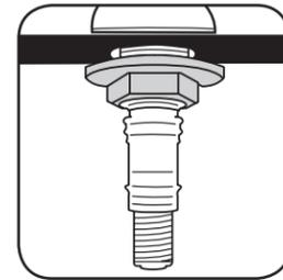
3. From below deck, use nut and metal washer to secure spout to deck. Hand tighten.
