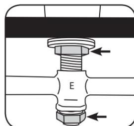
10. With a wrench, tighten center lower nut on shank and upper center nut.
