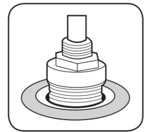
6. Above deck, place a sealing washer over each handle stem and around the cartridge housing.
