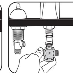
9. Align the undermount body (E) with deck holes and shank. Push the center of the undermount body onto shank. Be careful not to pinch o-rings.
