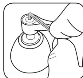
11. Install handles, connect water lines, and flush lines.
