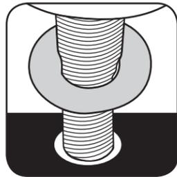
2. Slide the shank through the slim rubber washer and top center hole of deck.
