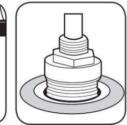
5. Above deck, place a sealing washer over each handle stem and around the cartridge housing.
