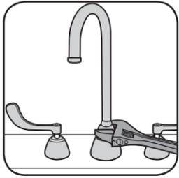
2. Place spout onto valve body until fully seated. Tighten spout nut with wrench. Connect water supplies, flush line, and attach outlet.
