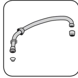
1. Remove outlet from spout. Place two split rings on spout tubing near base. Slide spout nut onto spout.
