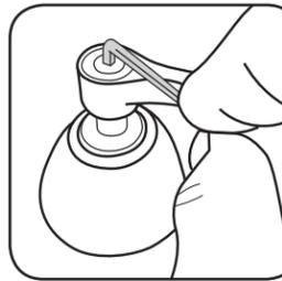
13. Install handles, connect water lines, and flush lines.
