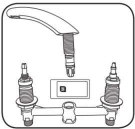
1. Using grease from supplied packet, lubricate the 4 o-rings on the spout shank and inside of center hub of undermount body.
