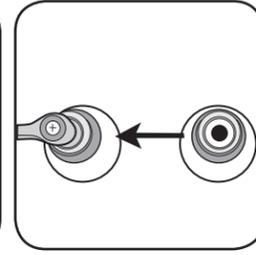
2. Place restricted swing body adaptor into valve body and align with internal valve body tab. Position small opening (70°) or large opening (120°) toward "hot" side of body.
