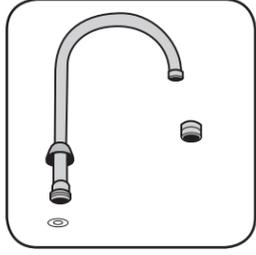
1. Remove outlet from spout. Slide spout nut onto spout. Place solid white washer into base outlet.
